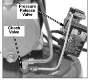
pressure release valve allows the motor to restart freely. When the motor stops running, air will be heard escaping from this valve for a few seconds. No air should be heard leaking when the motor is running, or continuous leaking after unit reaches "cut-out" pressure.
